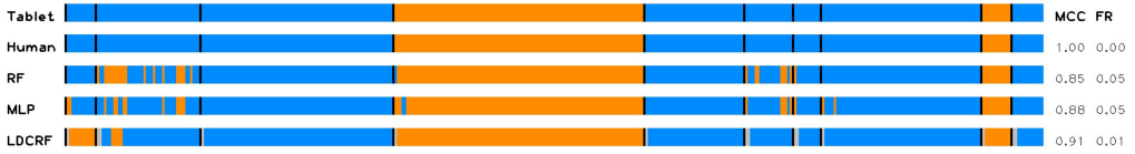
Fig. 10. Example timeline of a trial with the tablet ground truth, the human annotations, and the model predictions. Orange shows uninterruptible (0) while blue shows interruptible (1); gray indicates that there was insufficient data for the model to make a classification. Black indicates breakpoints between different moments of observation by the robot during the course of the trial.
