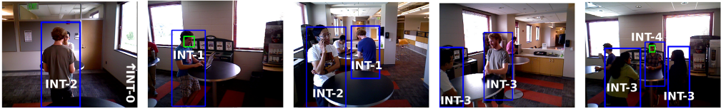
Fig. 3. Example scenes from the five data collection runs in the dataset in Section 6.2. The blue bounding box denotes individuals identified in the scene and the green bounding box denotes a face identified by the face recognition component. The interruptibility label of the identified individuals is also shown.
